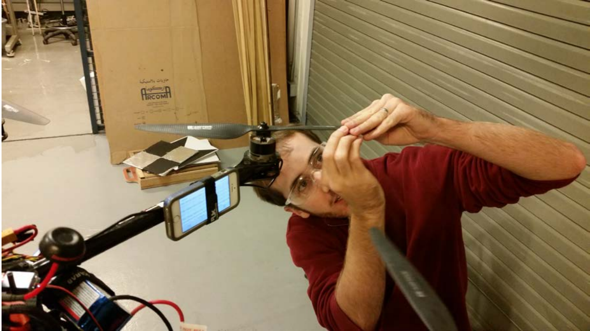
Figure 37 – Rebalancing UAV propellers using an iPhone accelerometer
