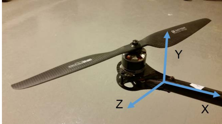
Figure 23 – Shrink-wrapped accelerometer installed on hexacopter arm, with sensor coordinate axes indicated [41]
