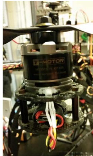
Figure 32 – a.) One Wire Digital Temperature Sensor DS18B20 [50] b.) Temperature sensor installed on UAV motor with thermal epoxy
